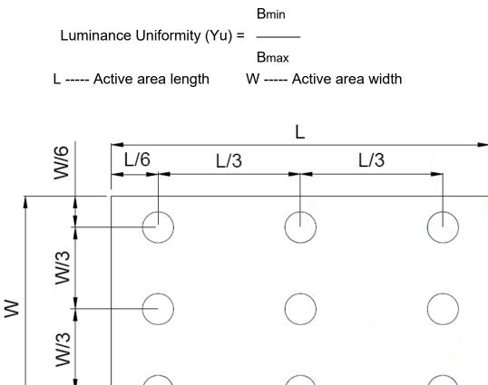
Bmax : The measured maximum luminance of all measurement position.Bmin : The measured minimum luminance of all measurement position.
